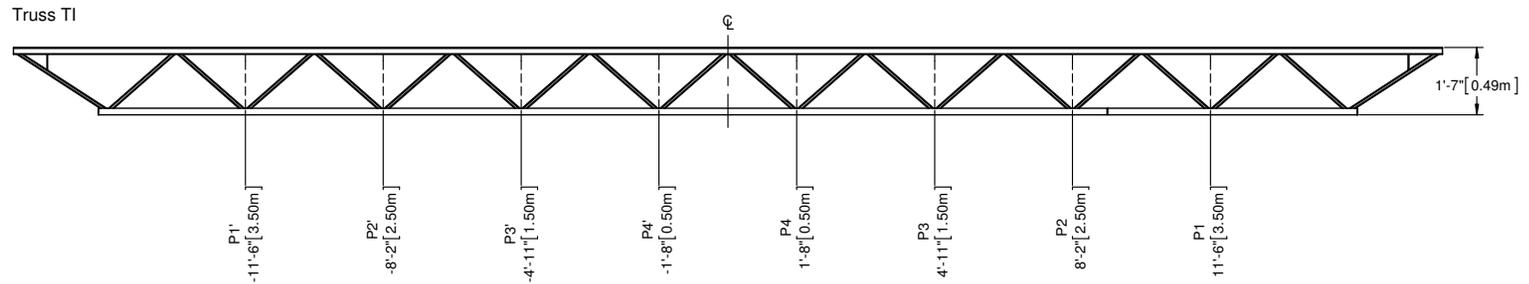
$$\text{Truss T1}^{**}: \frac{\text{Load P1}}{\text{Capacity P1}} + \frac{\text{Load P2}}{\text{Capacity P2}} + \frac{\text{Load P3}}{\text{Capacity P3}} + \frac{\text{Load P4}}{\text{Capacity P4}} \leq 1.00$$
