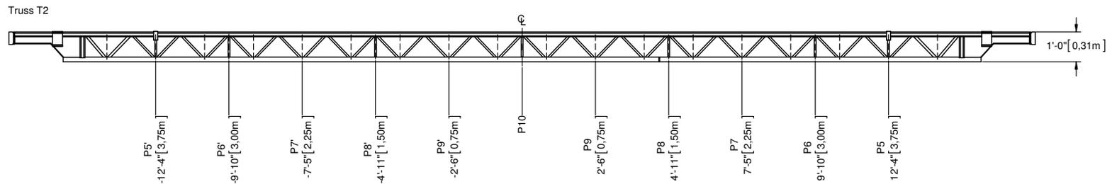
$$\text{Truss T2}^{**}: \frac{\text{Load P5}}{\text{Capacity P5}} + \frac{\text{Load P6}}{\text{Capacity P6}} + \frac{\text{Load P7}}{\text{Capacity P7}} + \frac{\text{Load P8}}{\text{Capacity P8}} + \frac{\text{Load P9}}{\text{Capacity P9}} + \frac{\text{Load P10}}{\text{Capacity P10}} \leq 1.00$$
